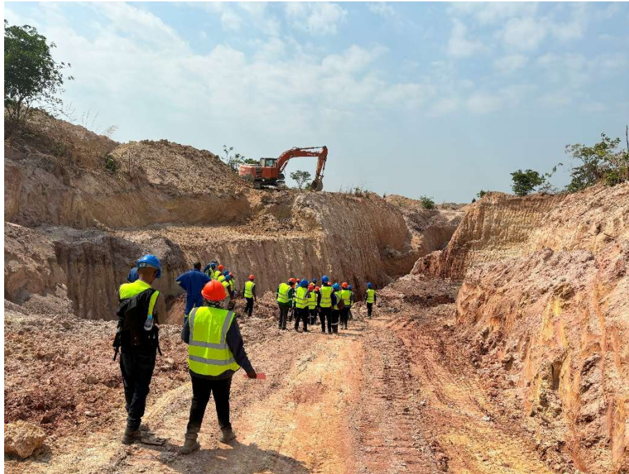
Figure 28. Small-scale open pit benched mine excavating manganese ore. Note the structural ramps designed for entry and exit. Source: Robin Gilli
